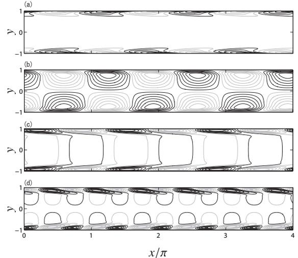
Figure 5: Contour plots of disturbance components by the traveling wave for  $c = 0.27$  and  $k = 1.5$ ; (a)  $T'$ , (b)  $v'$ , (c)  $u'$  and (d)  $-u'v'$ . The line increments are 0.15, 0.001, 0.005 and 0.00002 for  $T'$ ,  $v'$ ,  $u'$  and  $-u'v'$ , respectively. The black is the positive value and gray is the negative value.
