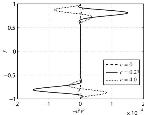
Figure 4: Profile of the Reynolds shear stress at  $k = 1.5$ ,  $\text{Re} = 2000$  and  $\text{Ri} = 0.0945$ .
