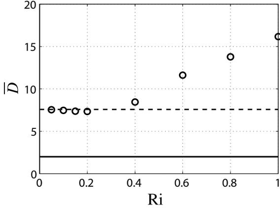
Figure 7: Time-averaged skin-friction drag,  $\bar{D}$ , as a function of the Richardson number,  $Ri$ , at the fixed wavenumber and wavespeed,  $k = 1.5$  and  $c^+ \approx 32$ , respectively. Broken line, uncontrolled level; solid line, laminar level.
