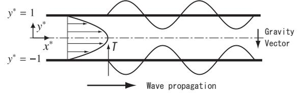
Figure 2: Flow geometry, coordinate system and the traveling wave-like surface heating/cooling as the control input.
