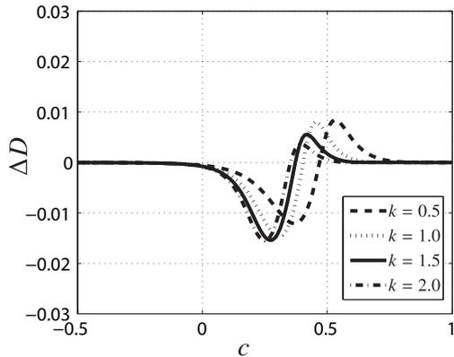
Figure 3: The drag increment,  $\Delta D$ , as a function of wavenumber,  $c$ , at  $\text{Re} = 2000$  and  $\text{Ri} = 0.0945$ .
