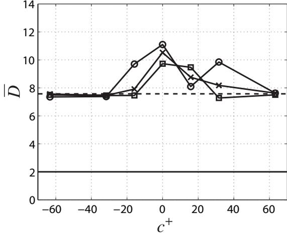
Figure 6: Time-averaged skin-friction drag,  $\bar{D}$ , as a function of wavenumber,  $c^+$ , in turbulent channel flow at  $Ri = 0.2$ :  $-\circ-$ ,  $k = 0.5$ ;  $-\times-$ ,  $k = 1.0$ ;  $-\square-$ ,  $k = 1.5$ ; broken line, uncontrolled level; solid line, laminar level.
