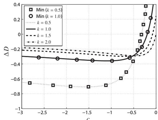
Figure 1: The drag increment,  $\Delta D$ , as a function of wavenumber,  $c$  by the traveling wave-like surface blowing/suction control of Min et al. (2006) reproduced by Mamori et al. (2008). The Reynolds number is  $\text{Re} = 2000$  and the waveamplitude of the traveling wave is  $a = 0.1$ .
