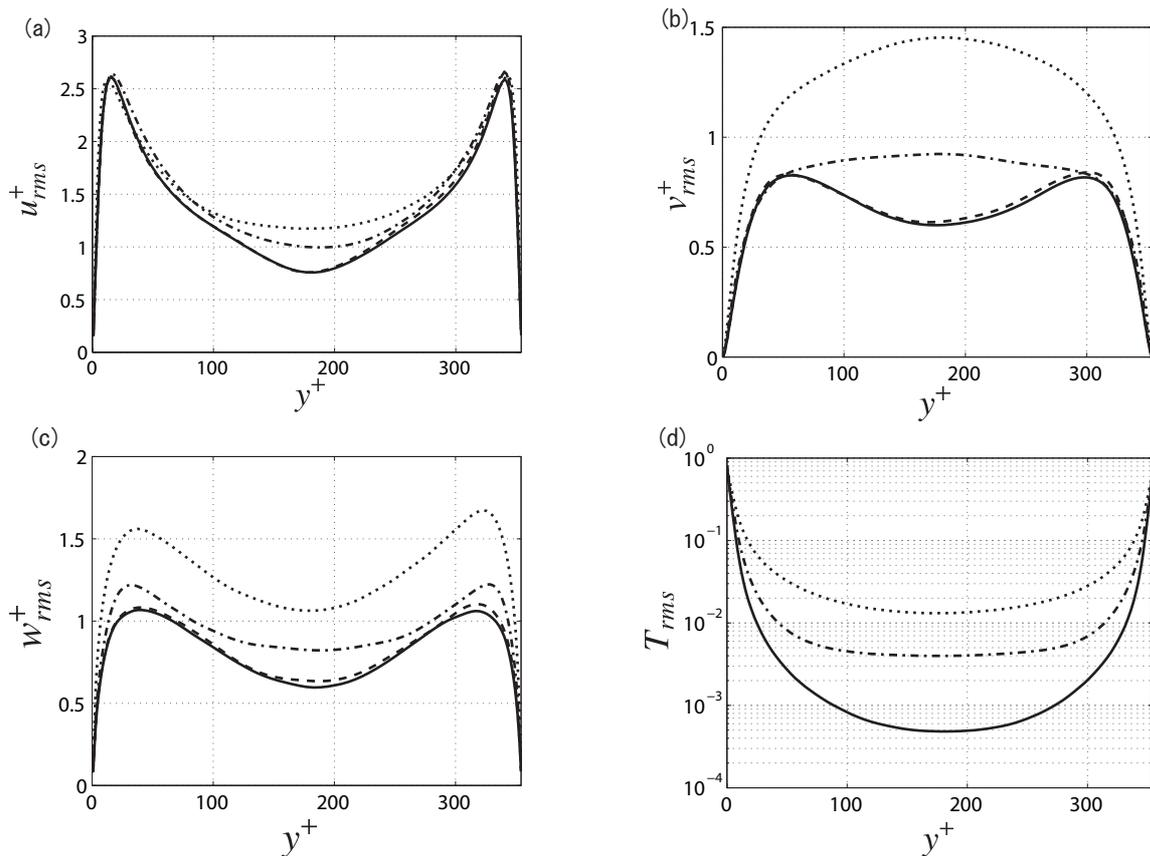
Figure 10: Profiles of the root-mean-square components at  $c^+ \approx 31$  and  $Ri = 0.2$ ; (a) streamwise velocity, (b) wall-normal velocity, (c) spanwise velocity, (d) temperature. The lines are the same as Fig. 8.
