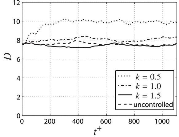
Figure 8: Time history of the skin-friction drag,  $D$ , by the different wavenumber compared with the uncontrolled flow.
