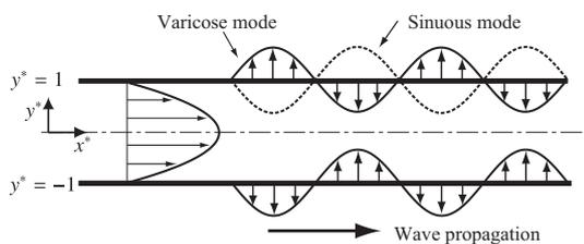
Figure 1: Flow geometry and schematic of control input.
